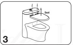
Remove the seat by unscrewing the toilet seat bolts from the hinges.
