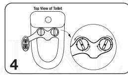
Place the bidet on the toilet. The plates may be adjusted depending on where the two holes on the back of the toilet are.
