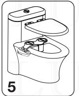
The bidet should now be aligned with the coupling holes.
