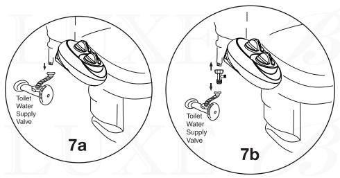
**Tip:** Do not use excessive force while tightening the connection. Hand tighten then use a wrench to gently tighten one quarter or a half-turn more.
