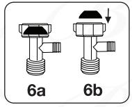
**6a:** Make sure that there is a black rubber washer inserted at the top of the t-adapter. **6b:** If it is not already there, insert it as shown in figure 6b.
